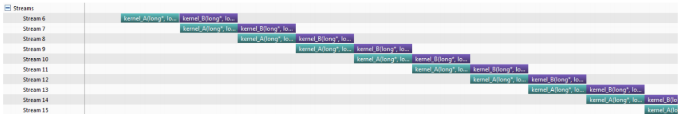
Figure 4: Profiling of older multi-engine GPUs without Hyper-Q
